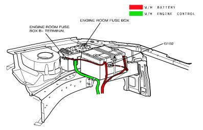
W/H ENGINE CONTROL MAT-TPS -IAC CAM SENSOR G104 CCCP SOLENOID LEGR DIS MODULE -ENGIN COOLANNT TEMPERATURE SENDER UNIT 0 CTS W/H Or SENSOR OIL PRESSURE G106 MAP ENGINE FUSE RELAY BOX NSBU ATM CONNECTOR
